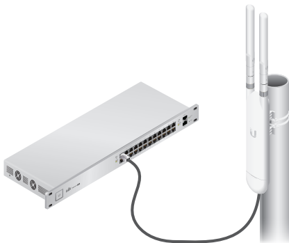
Connected to UniFi Switch, model US-24-250W
