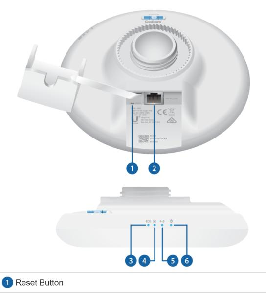
To reset to factory defaults, press and hold the Reset button for more than 10 seconds while the device is powered on. Alternatively, the device may be reset remotely via a Reset button located on the bottom of the Gigabit PoE Adapter.
