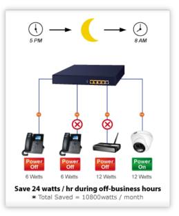
\_\_\_\_\_\_\_ 1000BASE-TX UTP with PoE
