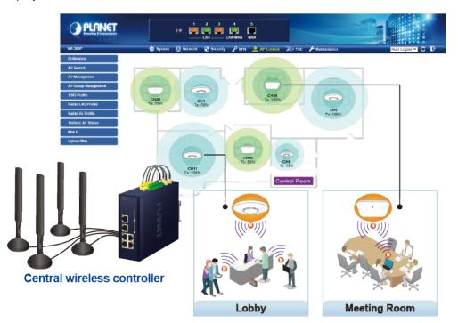
For example, to configure multiple Smart APs of the same model, the VR-300W5 allow clustering them to a managed group for unified management. According to requirements, wireless APs can be flexibly expanded or removed from a wireless AP group at any time. The AP cluster benefits bulk provision and bulk firmware upgrade through single entry point instead of having to configure settings in each of them separately.
