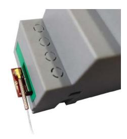
Connect the small antenna or pigtail before inserting it into the slot. Due to the limited space, this is much more complicated afterward.
