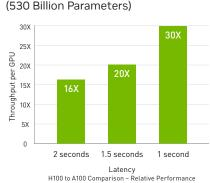
Projected performance subject to change. Inference on Megatron 530B parameter model chatbot for input sequence length=128,output sequence length =20 | A100 cluster: HDR IB network | H100 cluster: NDR IB network for 16 H100 configurations | 32 A100 vs 16 H100 for 1 and 1.5 sec | 16 A100
