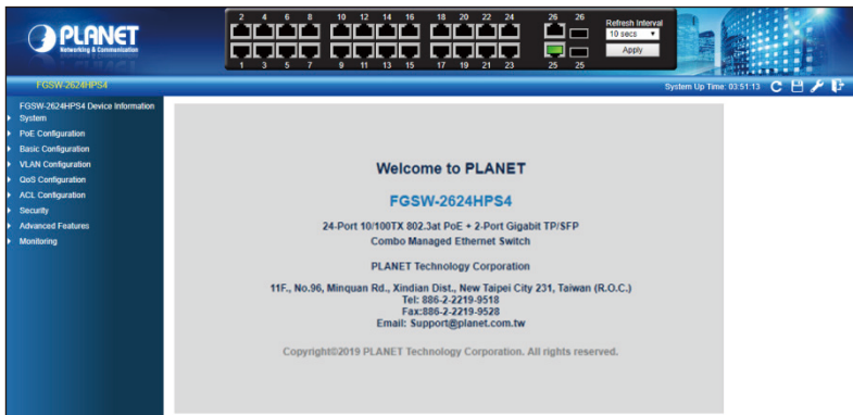
Figure 3-3: Web Main Screen of Managed PoE Switch
